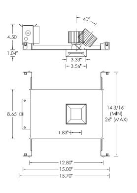
NC - New Construction Housing (Non-IC and CP rated) IC - New Construction IC Housing (2200lm max)
