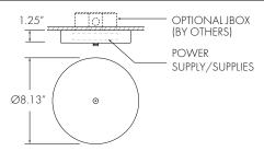
Surface mounted canopy with integrated 90.0 W driver with dimming. Available with dual circuit option. Dual option includes two seperate 90.0 W drivers.
