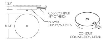
Surface mounted canopy for non-accessible ceilings with integrated 90.0 W driver ready for 0.5" conduit.
