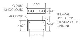
Remote power supply enclosure with 90.0 W driver with dimming. Plenum rated option available. (PL120 or PL277). Powder coated textured white.
