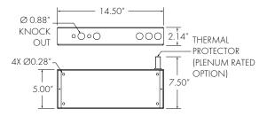
Remote power supply enclosure which includes  $2x\,90.0\,\mathrm{W}$  drivers with dimming. Provided with 96" HO fixtures. Provided with 72" and 96" SHO fixtures. Provided with all D10 fixtures. Plenum rated options available (PL120/PL277). Powder coated textured white.
