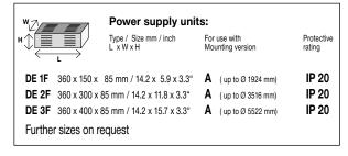
Input voltage for all external power supply units and canopy is 90-277 VAC 47-63 Hz
