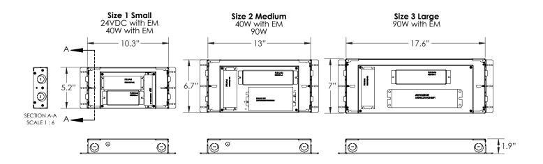
BBUX - BATTERY BACK-UP & LED DRIVER REMOTE (OUTDOOR), IP67, IK10, NEMA 4X, -20°C to +55°C, 30' MAX Distance with 12AWG (w/UNV Option Only)
