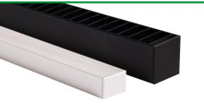
Utilizing a clear lens that sits flush to the fixture housing, the VERS Insert is a finished aluminum fixture whose lens profile allows for the insertion of a film. Insert includes a batwing or prismatic for glare reduction while disguising the LED diodes. Integrated metal endcaps combined with an extruded aluminum housing in satin, black, bronze or white finishes are available and can be installed in dry, damp, and wet locations for controlled lighting in any setting.
