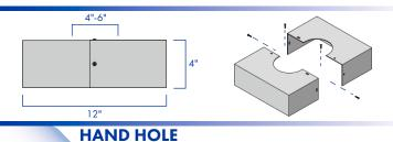
HAND HOLE: Reinforced 3" x 5" hand hole is located 18" above base. Cover and attachment hardware provided.
