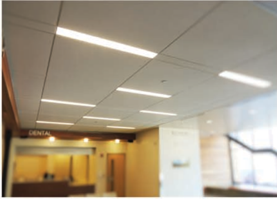
Flush with 15/16" grid (T1W)
