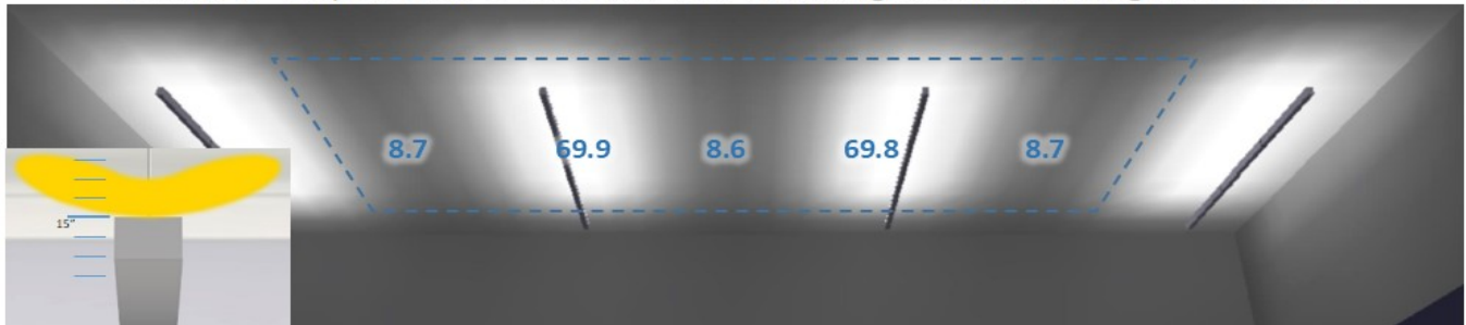
GGMS, 15" suspension, 14' on center row mounting, max\min ceiling ratio of 8.13:1
