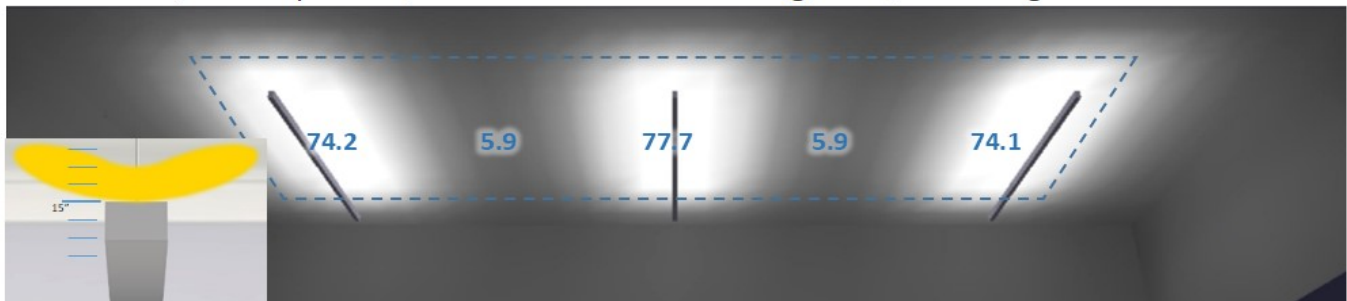
GGMS, 15" suspension, 16' on center row mounting, max\min ceiling ratio of 13.17:1
