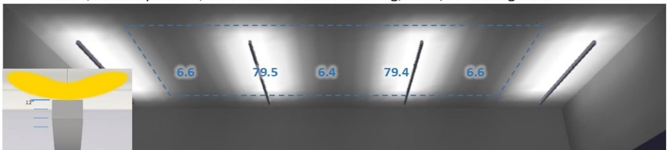
GGMS, 12" suspension, 14' on center row mounting, max\min ceiling ratio of 12.42:1
