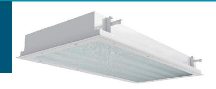
**Application:** The Vyv VSCRU Cleanroom Recessed Universal Luminaire is certified IP65 and rated for ISO Class 3-8 cleanrooms. The inset door seals directly to the housing and overlapping door seals to the ceiling and housing, completely covering the fixture flange. Triple gasketed, listed for wet locations and is tested to 2500Psi washdown. Inset door suitable for Biosafety BSL1-2 and overlapping door for BSL1-3.
