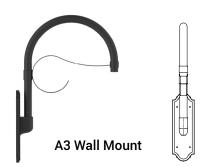
Architectural Arm 3 is constructed of extruded aluminum tubing. Integrates with poles or tenons of 3-1/2", 4", 4-1/2", or 5" OD and is secured with 3/8" stainless steel Allen set screws.
