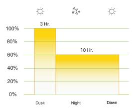
Time & dimming settings are set with the remote solar charger programmer
