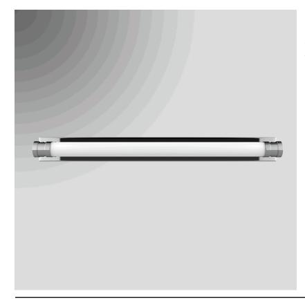
50" LED Ready Chrome Vanity Fixture, direct wired, Frosted White Glass Diffuser. Recommend one 15 watt T8 LED linear Non-Shunted bulb (bulb not included, fixture will not work with a fluorescent bulb)
