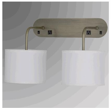
17"H Brushed Brass Pendant, two medium base sockets, two independent on/off rocker switches, two outlets,8' Silver 45° 3-prong grounded cord to exit back of lamp, 2-10x10x8 White Linen HB Shade with bottom diffuser. Recommend 2-1100 lumen LED bulbs.
