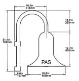
General: The classic straight-shade design of the Epic series provides a full-cutoff decorative fixture. Fixture was designed to meet IESNA standards for full-cutoff, eliminating upward light pollution.
