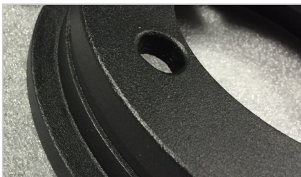
extruded bollard tube slides over cast aluminum mounting base and secures to base with (4) set screws tightened into machined groove
