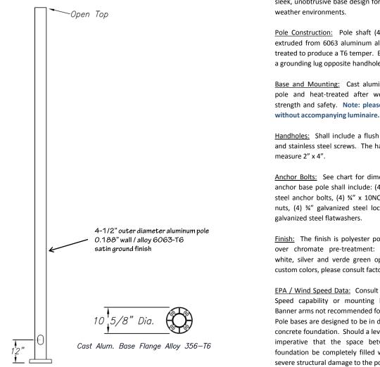
(4) 3/4"-10NC Galv. Stl. Anchor Bolts, ÀÁSHÍO M314—90 Grade 55, 10" Of Threaded End Galv. Per ASTM A153. (4) 3/4"–10NC Galv. Stl. Hex. Nuts (4) 3/4" Galv. Stl. Lockwashers (4) 3/4" Galv. Stl. Flatwashers
