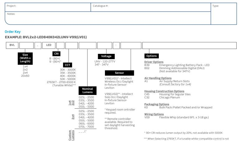
\*\*\* When Selecting 2765KT, if a tunable white-compatible control is not selected the luminaire will come standards with two sets of 0-10V wires for dimming and color tuning (see tunable white diagram for details). For compatible control options please consult factory.
