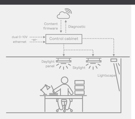
In larger installations the NatureConnect system can be integrated with an external lighting control system.
