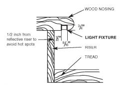
Custom fabricated fixtures are manufactured to the exact. dimension required. Each LED fixture is built with an 18" lead wire from one end. NOTE: various fixtures permit the client to specify from which end the lead wires exit. The maximum fixture length for any type is 15 feet (180 inches.) (Please consult with an RSL representative for solutions on extra-long lengths.) When pricing, always round up to the nearest half foot.
