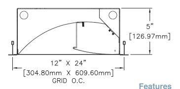
Durable steel housing with perforated side basket.
