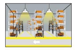
If there is no motion detected, the light will be remained at a low light level all the time.
