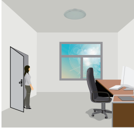
1. No motion detected, all lamps switch off.
