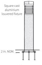
(4) ½ in. X 12 in. Galv. Steel Anchor Bolts W/ Washers Astm F1554 Grade 36
