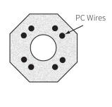
Shaft cross section detail
