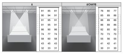
Footcandle calculations based on standard reflectance of 90/60/30 and a light loss factor of 1.0. Fixtures spaced 3' 6" O.C. over 3' wide bed at an 8' ceiling height. Values are for bed surface.
