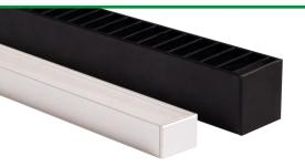
The wet rated VERS Encapsulated (06) is a finished aluminum fixture that is fully encapsulated in polyurethane and suitable for use in various applications. Encapsulation is available in a clear finish where diodes are visible or a translucent finish, for diffused light. The internal WhiteOptics® technology combined with the polyurethane encapsulation provide optimal delivered lumens.
