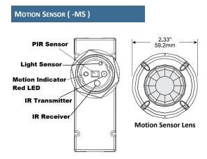
PIR Motion Sensor (120v-277v only) option includes (1) passive infrared (PIR) sensor to detect motion. When motion is not detected for a 3-1/2 minute period, luminaire will automatically dim to 20% power and light. Once motion is detected, luminaire immediately ramps up to 100% power and light output until motion is not detected for another 3-1/2 minute period.
