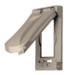
Recessed receptacle outlet box mounted 16" on center from bottom of bollard tube. Cast aluminum outlet box internally welded and sealed with gasketed spring-loaded hinge cover. Cover shall be die cast metal construction with finish to match bollard.
