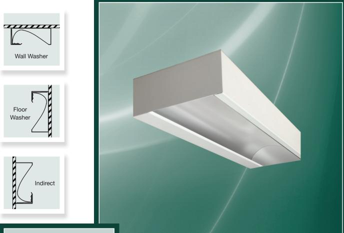
Ideal placement is 24" to 36" from the front edge of fixture to the surface you are lighting, for 8' to 12' ceilings.
