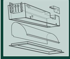
Ideal placement is 8" to 12" from the front edge of the fixture to the surface you are lighting, for 8' to 10' ceilings.
