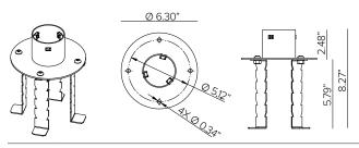
Powder coated mounting base with ground anchor fixing rods for installation in concrete. AISI 316 stainless steel. Mounting bolts included. **Required for use with 1US2530 by NEC.**
