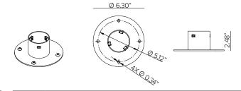
Powder coated mounting plate for surface installation outside the post. AISI 316 stainless steel compatible with dowels to be inserted into 4 holes, Ø 0.34" Dia. for use with 5/16" bolts maximum. Anchor bolts not included. **Required for use with 1US2530 by NEC.**
