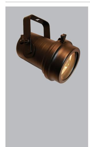
The MK3 is an ideal fixture for highlighting artwork, exhibits, and retail displays. This unit accepts low voltage AR111 lamps in a variety of beam spreads. The MK3 features a hinged front for easy re-lamping and has the ability to accept louvers, barndoors, hoods and a variety of filters.
