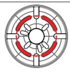
6.5" bolt circle for Drilled Anchors. Used when existing anchor bolts do not fit 4-bolt or 3-bolt slot or are damaged. these must be cut off and new drilled anchors installed
