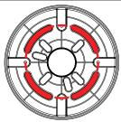
6.5" bolt circle for Drilled Anchors. Used when existing anchor bolts do not fit 4-bolt or 3-bolt slot or are damaged. these must be cut off and new drilled anchors installed
