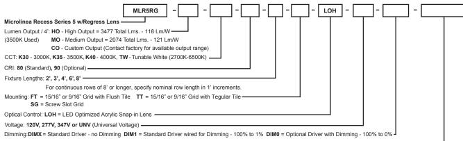
Options: NLCKT = Night-Light Circuit (Common Neutral) EMCKT = Emergency Circuit (Separate Hot & Neutral) EBPHST = Self-Test Emergency Battery Pack (10 Watt)-**DALI** = DALI Protocol Driver (Tunable White) **DMX** = DMX Protocol Driver (Tunable White) **0-10V/TW** = 0-10V Driver (Tunable White)
