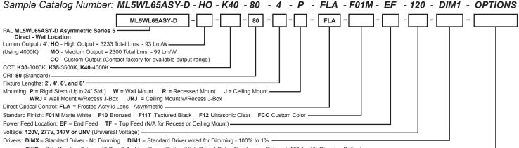
CWD = Cold Weather Driver, -40 Deg C Ambient Temp. Rating (High Output Only - 3' or Longer Fixtures) (N/A for 1% Dimming Option)
