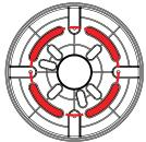
6.5" bolt circle for Drilled Anchors. Used when existing anchor bolts do not fit 4-bolt or 3-bolt slot or are damaged. these must be cut off and new drilled anchors installed
