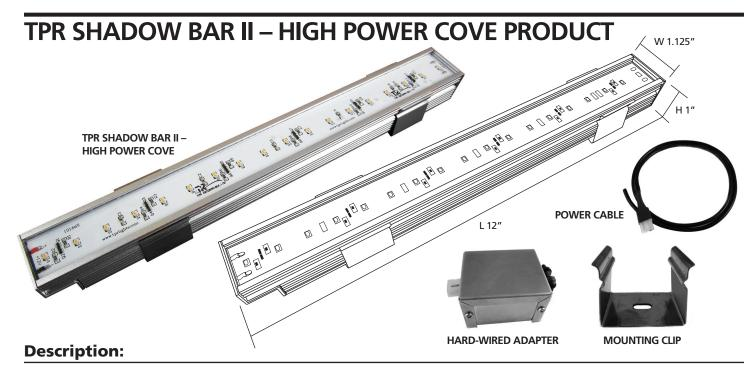
The TPR SHADOW BAR II is an energy efficient LED Linear cove product for Hospitality, Retail, Commercial and Residential use. It has extremely close binning, comes in several color temperatures and is fully dimmable. The Shadow Bar II has an extruded aluminum housing and is rated IP44 for indoor use.
