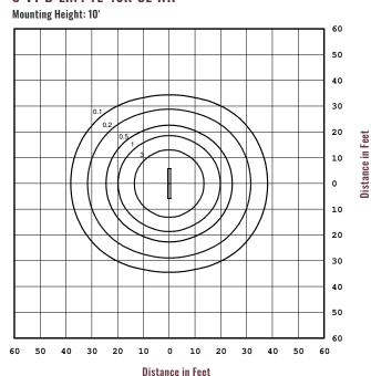
Note: All published photometric testing performed to IES LM-79 standards. Fixture photometry was completed on a single representative fixture. Foot candle levels are noted inside graph.
