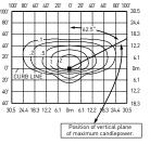
NTA-A-NM-T3-11L-40K-UL-BZ w/NTA-BLSF-11L Mounting Height: 25' (7.6m) A.F.G. Initial Delivered Lumens: 7,575 Initial FC at grade
