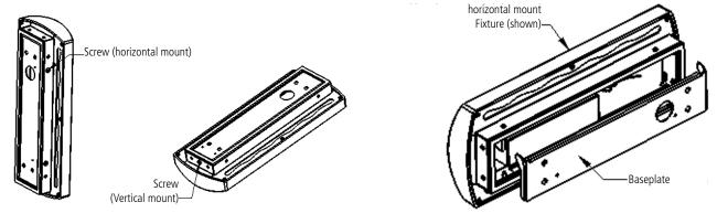
3. Mount baseplate. Use the baseplate as a template and mark the pilot holes on the mount surface. Orient the baseplate with the angle brackets hook at the top. Use 1/4-20 screws (supplied by others) and anchors appropriate for the mounting surface. Remember to use non-ferrous metals when installing MRI fixtures.
