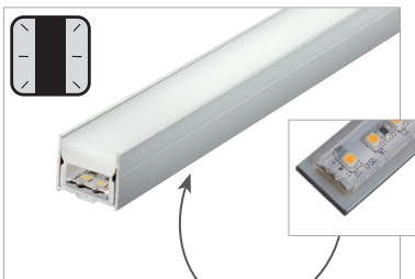
PRINTC-G Rigid high impact resistant PMMA profile complete with a white plastic diffuser lensed channel for recessed walk over installation. Complete with track for easy strip insertion. Available in 3.28ft (1M) lengths.
