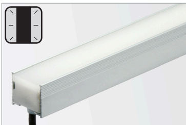
P03E-S-PF-300 Aluminum high impact walk over rated profile with white PMMA screen for recessed installation. Available in 118in (3M) lengths.
