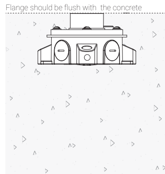
Box with Standard Flange: During Concrete Installation
