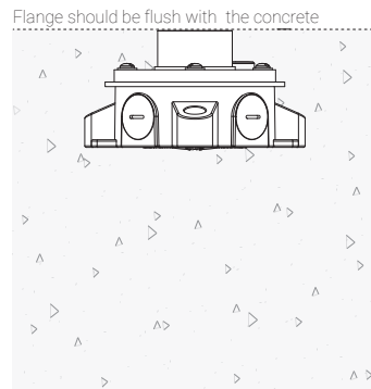
Box with Standard Flange: During Concrete Installation
