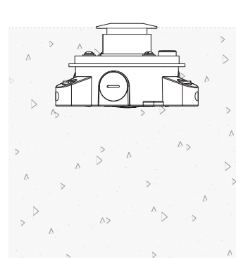
Box with Standard Flange: Complete Concrete Installation
