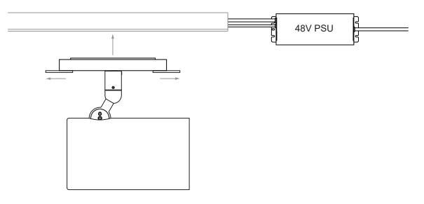
Pull out tabs to release locking grips and insert the adaptor into the track.
