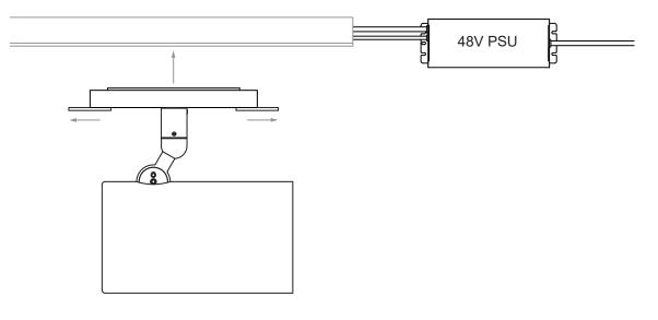
Pull out tabs to release locking grips and insert the adaptor into the track.
