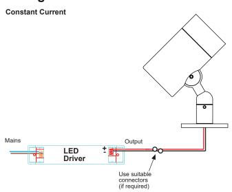
Note that while constant current light sources can be wired in series, the number of fittings that can be wired in series is limited by the forward Voltage of the LED.
