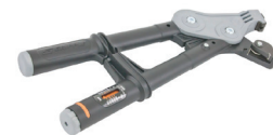
LS-TT Catenary Cable Tensioning Tool up to 880lbs with minimal effort due to the 6:1 gear drive mechanism. Integral torque gauge controls the load applied to the wire, giving consistent tension every time and optimizing the life of the wire.
